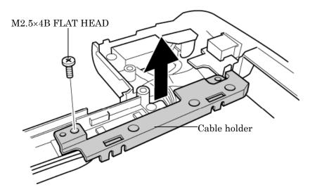
Figure 4-32 Removing the cable holder
